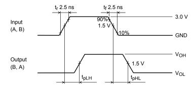
Figure 2 t<sub>pLH</sub>, t<sub>pHL</sub>
